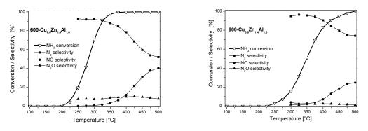
Fig. 1. Selective catalytic oxidation of ammonia over hydrotalcite derived catalysts
